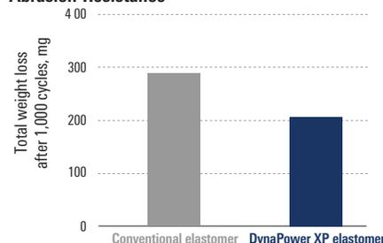
The DynaPower XP extreme-power motor elastomer operates three times longer, has a 10% higher pressure rating, and shows 30% more abrasion resistance than conventional elastomers.
