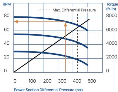
Power section differential pressure is the difference between "Off-Bottom" and "On-Bottom" pressure. Draw vertical line from corresponding pressure differential value to RPM curve and read motor speed on left axis. (Interpolate RPM for GPM values not shown on chart) Dotted line shows recommended maximum pressure can result in frequent stalling of motor and premature stator failure.
