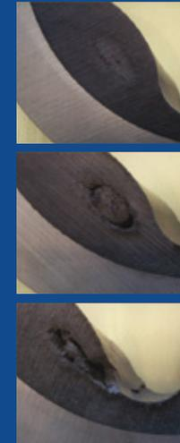
1. Hysteresis heat begins the degradation of the rubber in the middle of the stator
