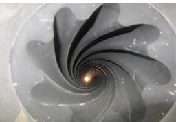
The DynaPower XR elastomer enabled the motor to sustain ROP and perform for 186 circulating hours at over 280 degF [138 degC], successfully drilling to TD in a single trip. During drilling, the ROP averaged 26.7 ft/h [8.1 m/h], which is a 20% improvement as compared with offset wells. The PowerDrive vorteX RSS with the DynaPower XR elastomer showed zero damage during the postrun check.
