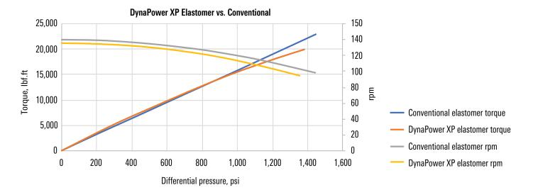
Data from lab tests indicated that the DynaPower XP elastomer produced the same power and torque output as the thin-wall power section lined with a conventional elastomer.
