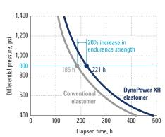
Data in the endurance strength graph was computed using Dyna-Drill proprietary 3D modeling software that took the following parameters into account: elastomer properties, stator and rotor geometries, downhole pressures and temperatures, mud properties, flow rate, and differential pressures.
