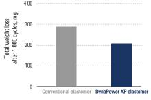
The DynaPower XP extreme-power motor elastomer operates three times longer, has a 10% higher pressure rating, and shows 30% more abrasion resistance than conventional elastomers.
